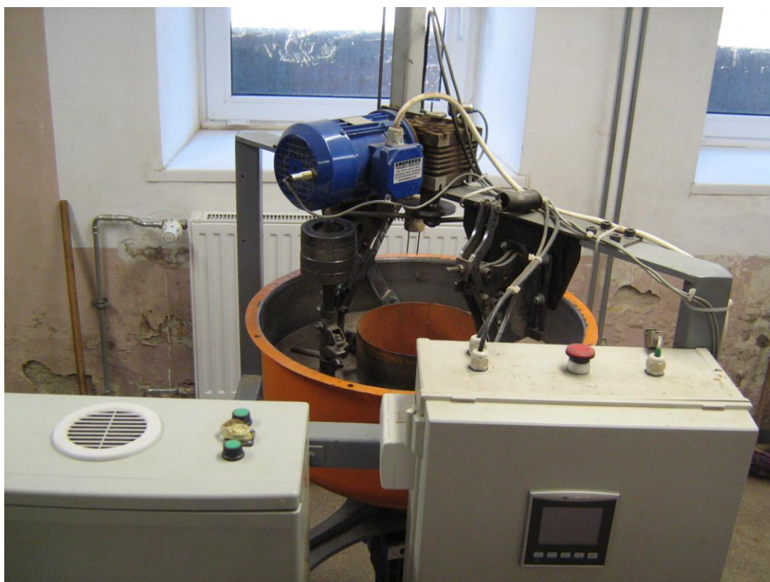
Fig. 4.1.75.2. View of the modernized 'rotating bowl' test rig intended for testing wear in soil (in the foreground control cabinets with inverters and software, in the background the mechanical part of the test rig)
