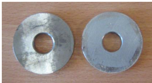
Fig. 4.3.3.10. Examples of disc-disc samples made of steel, intended for tribological tests on the SMC-2 test rig
