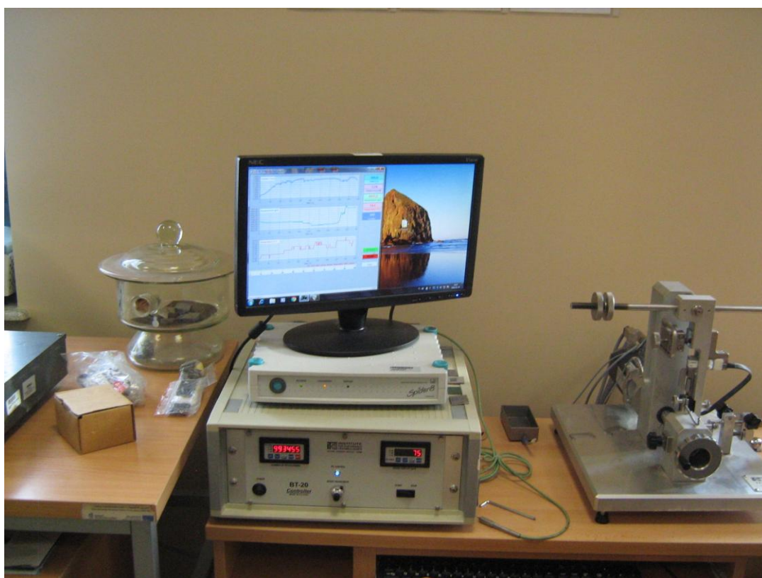
Fig. 4.1.74.4. A test rig of the ball-disc type consisting of a set of units: BT-20 controller, Spider 8 amplifier and T-20 tribotester
