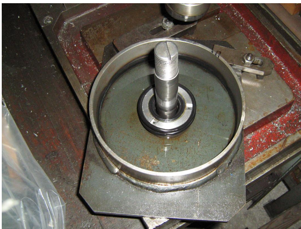
Fig. 4.1.9.24. The base plate of the test rig for tribological tests with a friction contact of conformal contact with visible three millings for samples
