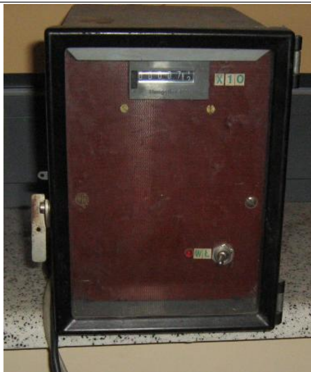
Fig. 4.3.3.5. The lower sample rev counter used in the original equipment of the SMC-2 tribotester
