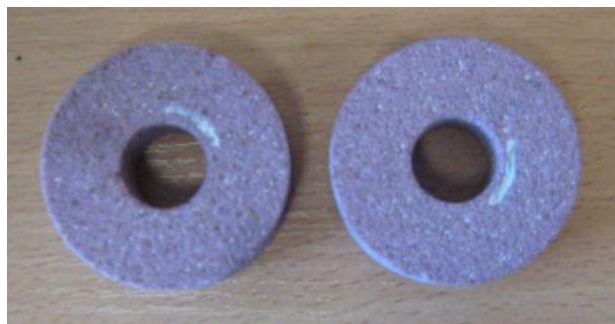
Fig. 4.3.3.11. Examples of disc-disc samples made of abrasive material bonded with a binder, intended for testing on the SMC-2 tribotester
