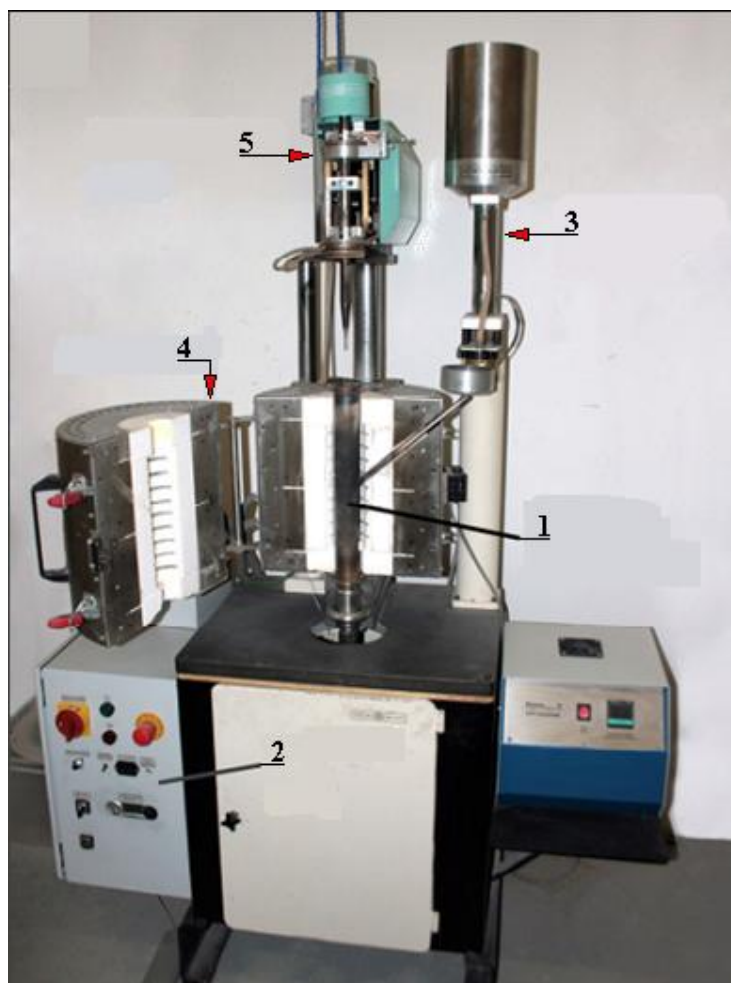
Fig. 4.1.82.3. A general view of the HT-CIAT tribotester 1 - test chamber, 2 - control cabinet, 3 - abrasive tank, 4 - thermal insulation, 5 - compressed gas medium supply unit
