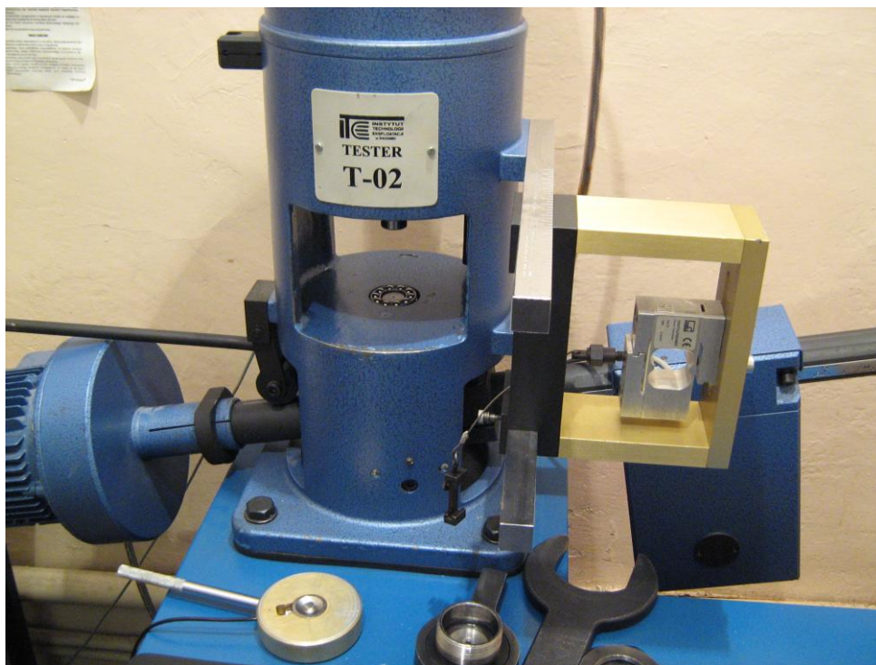
Fig. 4.2.6.4. View of the modernized T-02 four-ball test rig Visible change in the type of torque meter used. One of the military laboratories
