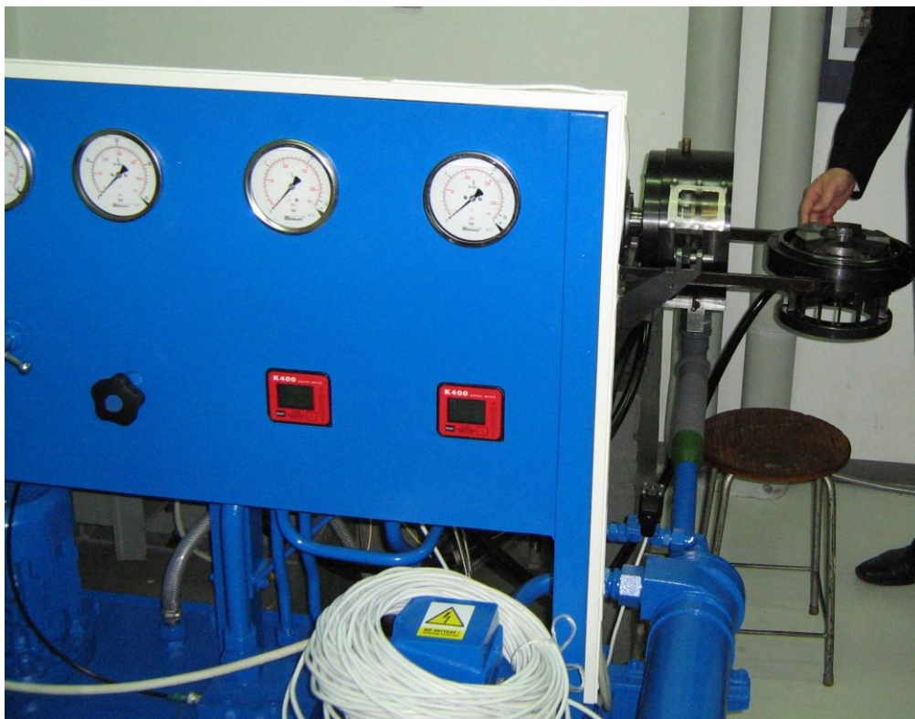
Fig. 4.1.18.3. The main panel of the hydraulic unit of the SON test rig with the visible disassembled thrust bearing tested
