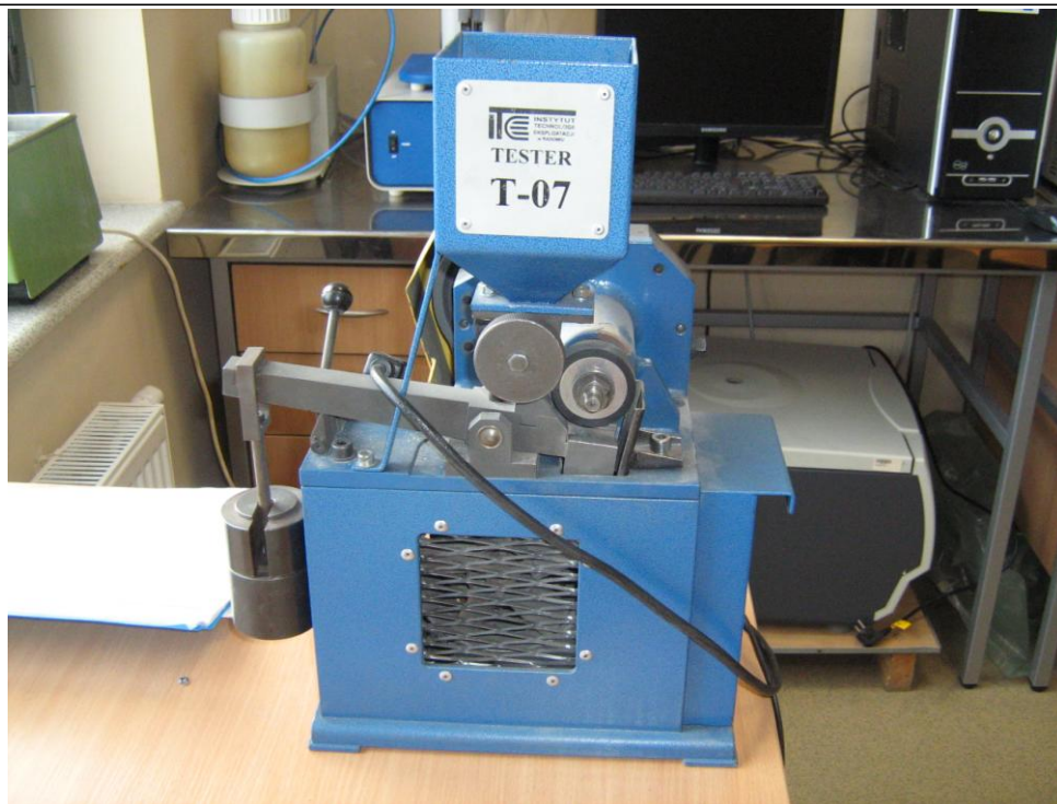
Fig. 4.1.73.4. T-07 abrasion test rig View from the side of the load contact
