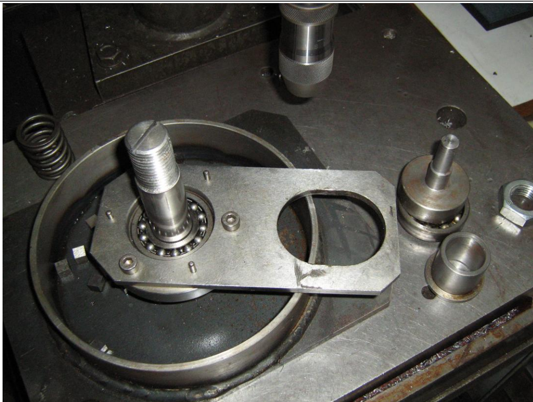
Fig. 4.1.9.27. A partially assembled test rig for tribological tests with a friction contact of conformal contact (mechanical part)
