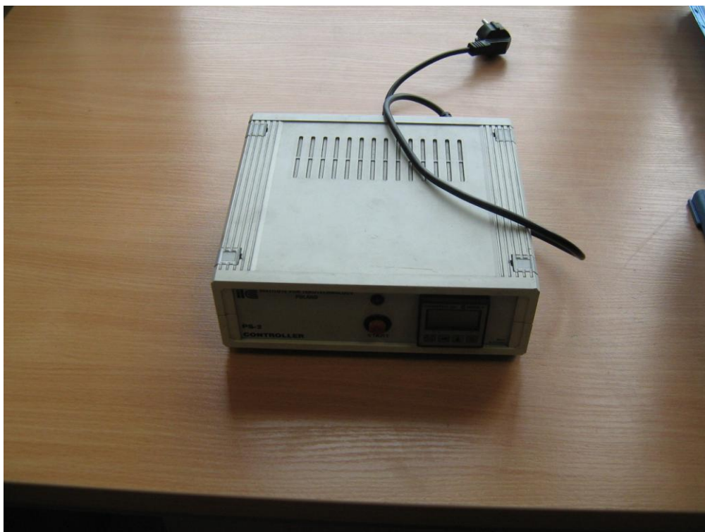
Fig. 4.1.73.13. The PS-2 Controller is used to program the operating parameters of the T-07 abrasion test rig
