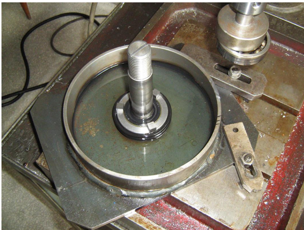
Fig. 4.1.9.23. The base plate of the test rig for tribological tests with a friction contact of conformal contact with visible 3 samples immersed in the oil chamber
