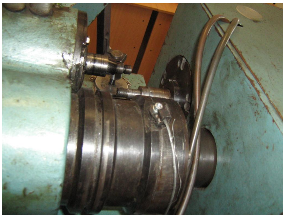
Fig. 4.3.3.6. In the foreground - a carriage drive shaft. In the far right - the lower sample drive shaft, on the left - the upper sample shaft
