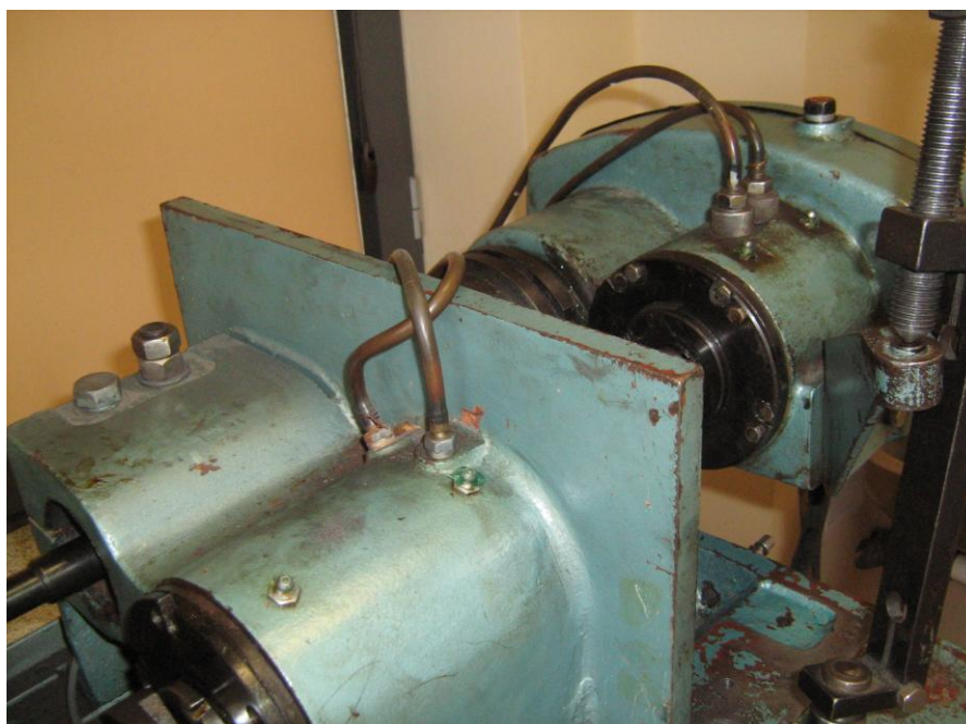
Fig. 4.3.3.8. Hoses of the carriage drive shaft cooling system and the lower sample headstock
