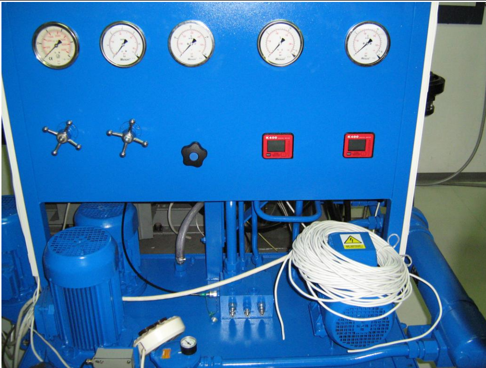
Fig. 4.1.18.2. The main panel of the hydraulic unit of the SON test rig
