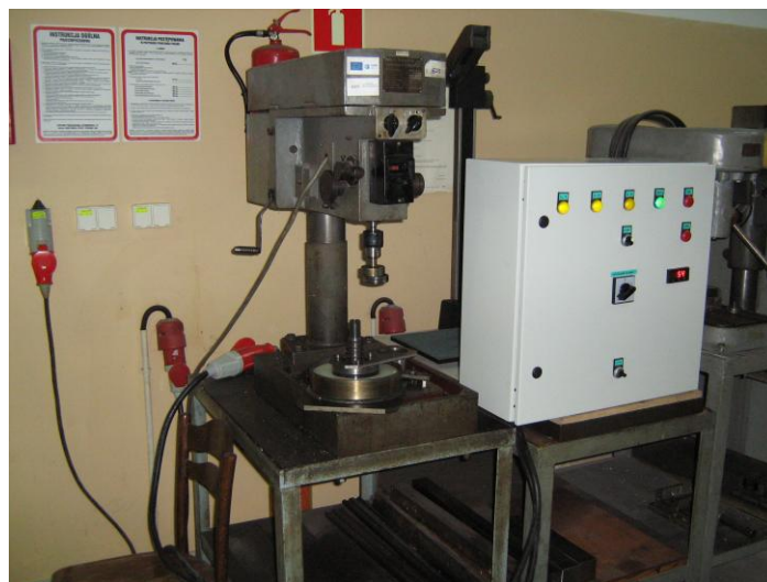
Fig. 4.1.9.22. Prepared test rig for tribological tests with a friction contact of conformal contact. Side view.
