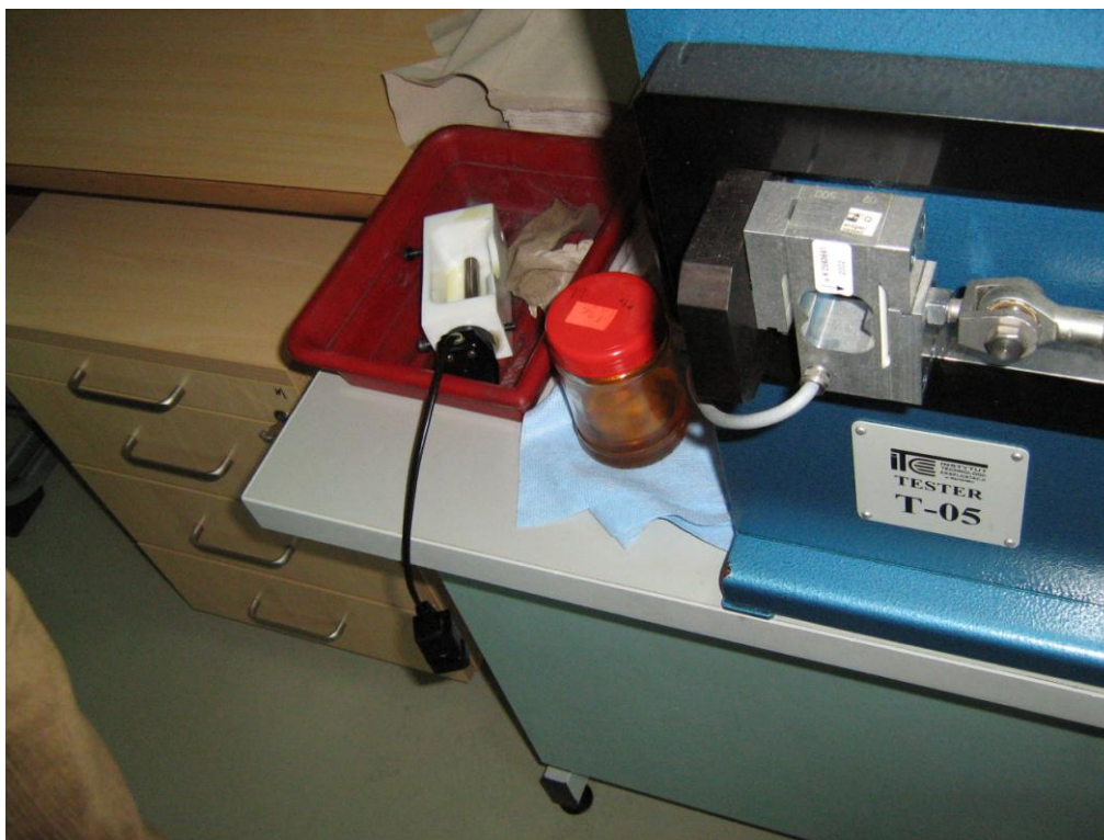
Fig. 4.2.2.2. Attachment for bath lubrication of test samples. T-05 test rig
