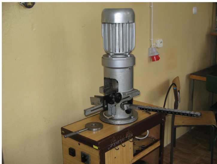
Fig. 4.3.1.13. General view of an exemplary four-ball test rig with a friction contact as in Figure 4.3.1.2.
