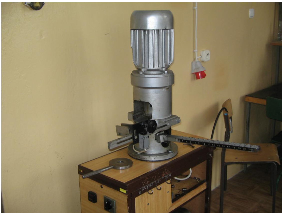
Fig. 4.2.16.1. An older type of a four-ball test rig designed to test the boundary friction. General view
