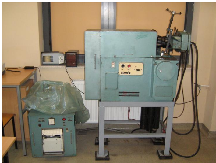
Fig. 4.3.3.1. A general view of the SMC-2 test rig (on the left side a control panel with the printer of the moment of friction)
