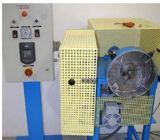
Fig. 4.1.82.2. A general view of the CIAT tribotester after removing the outer drum
