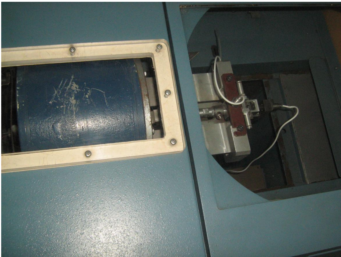
Fig. 4.1.15.3. FRET III test rig built at the Department of Construction and Operation of Machines, Faculty of Mechanical Engineering of Gdańsk University of Technology - visible, among others, displacement sensors, exciter
