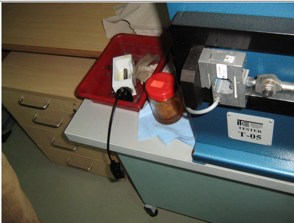
Fig. 4.2.2.2. Attachment for bath lubrication of test samples. T-05 test rig
