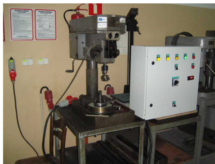
Fig. 4.1.9.22. Prepared test rig for tribological tests with a friction contact of conformal contact. Side view.
