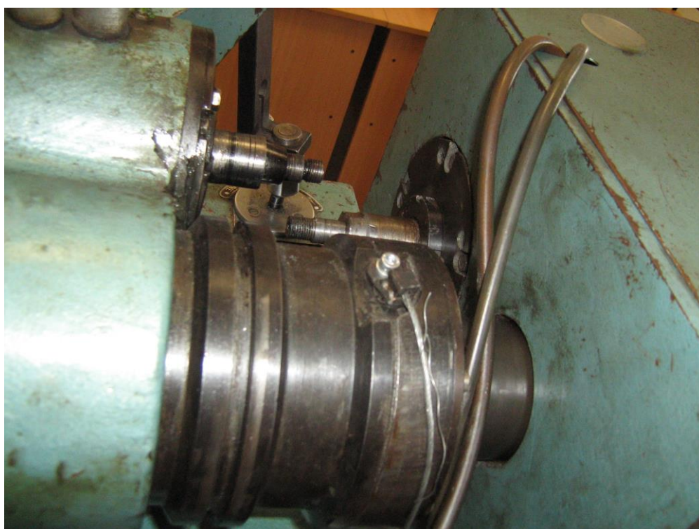
Fig. 4.3.3.6. In the foreground - a carriage drive shaft. In the far right - the lower sample drive shaft, on the left - the upper sample shaft
