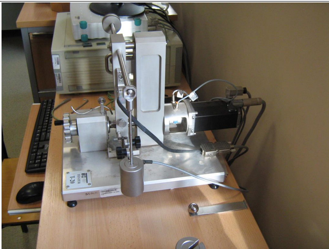
Fig. 4.1.74.5. T-20 tribotester (the view from the side of the load contact)
