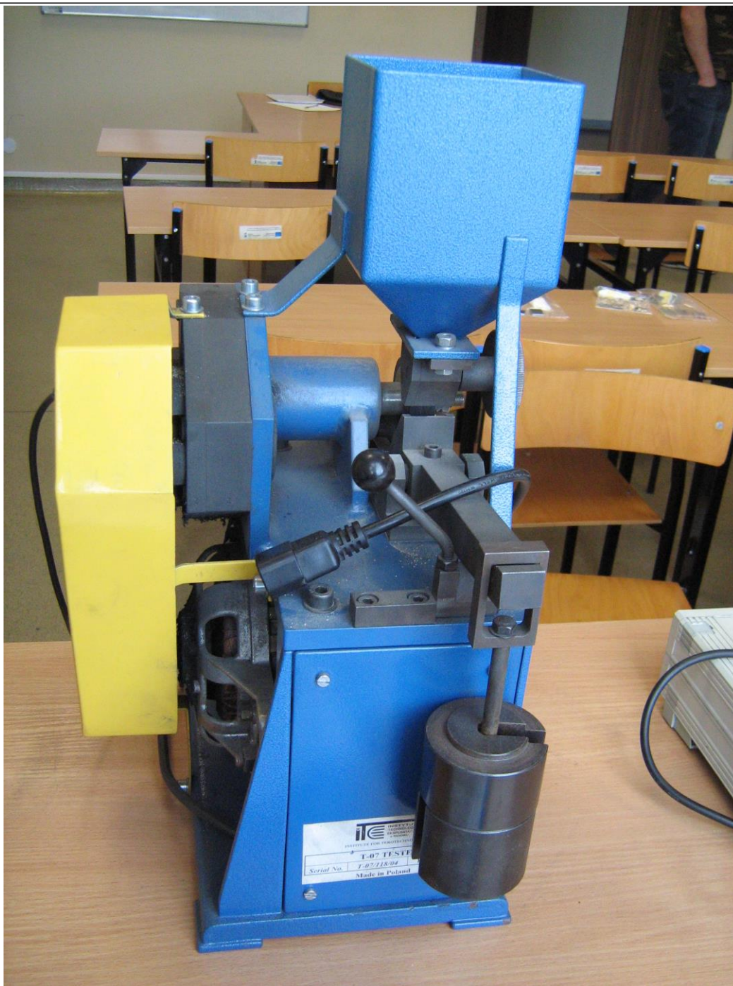
Fig. 4.1.73.6. T-07 abrasion test rig. Serial number T-07/118/04 from 2004. View from the side of the load unit
