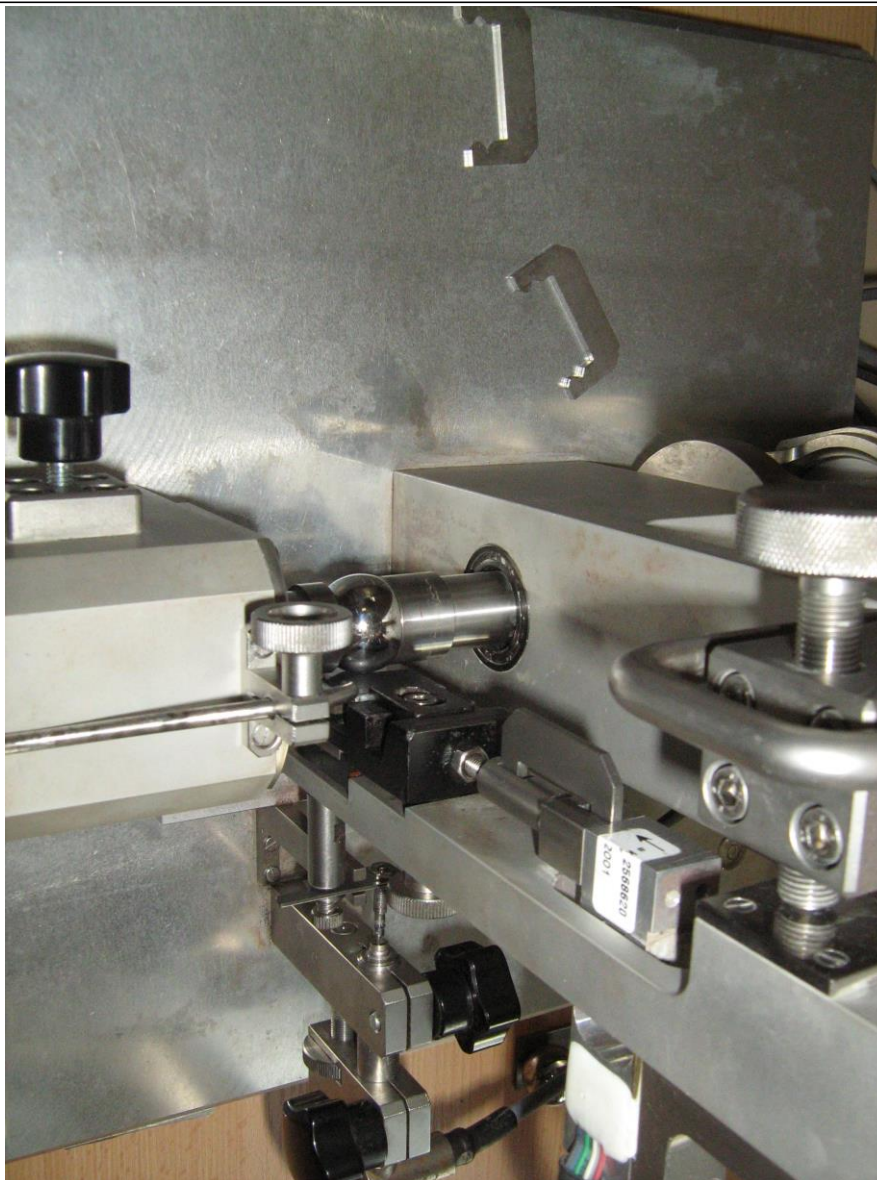
Fig. 4.1.74.6. The ball-disc friction contact used in the T-20 tribotester
