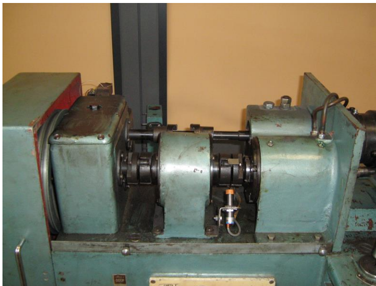
Fig. 4.3.3.3. A view of the carriage drive shaft after removing the cover. Visible pipes for cooling water supplied from the water supply system
