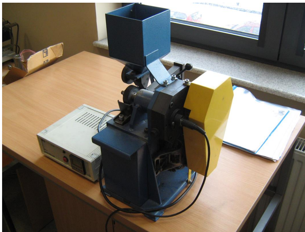
Fig. 4.1.73.5. T-07 abrasion test rig. Serial number T-07/118/04 from 2004. View from the drive side
