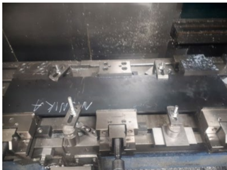
Fig. 27. Base plate mounted on a CNC milling machine
