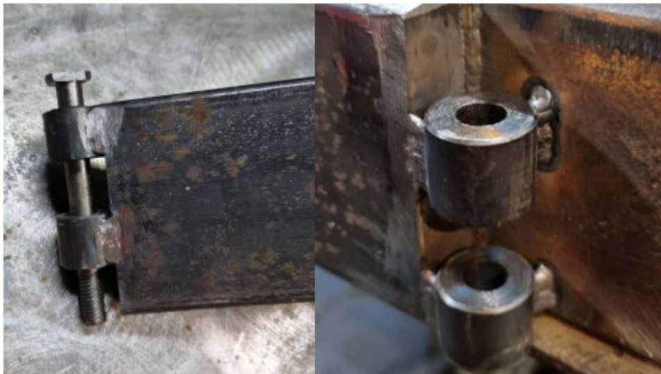
Fig. 34. Welding the bushing into the turntable arm and into welding table arm
