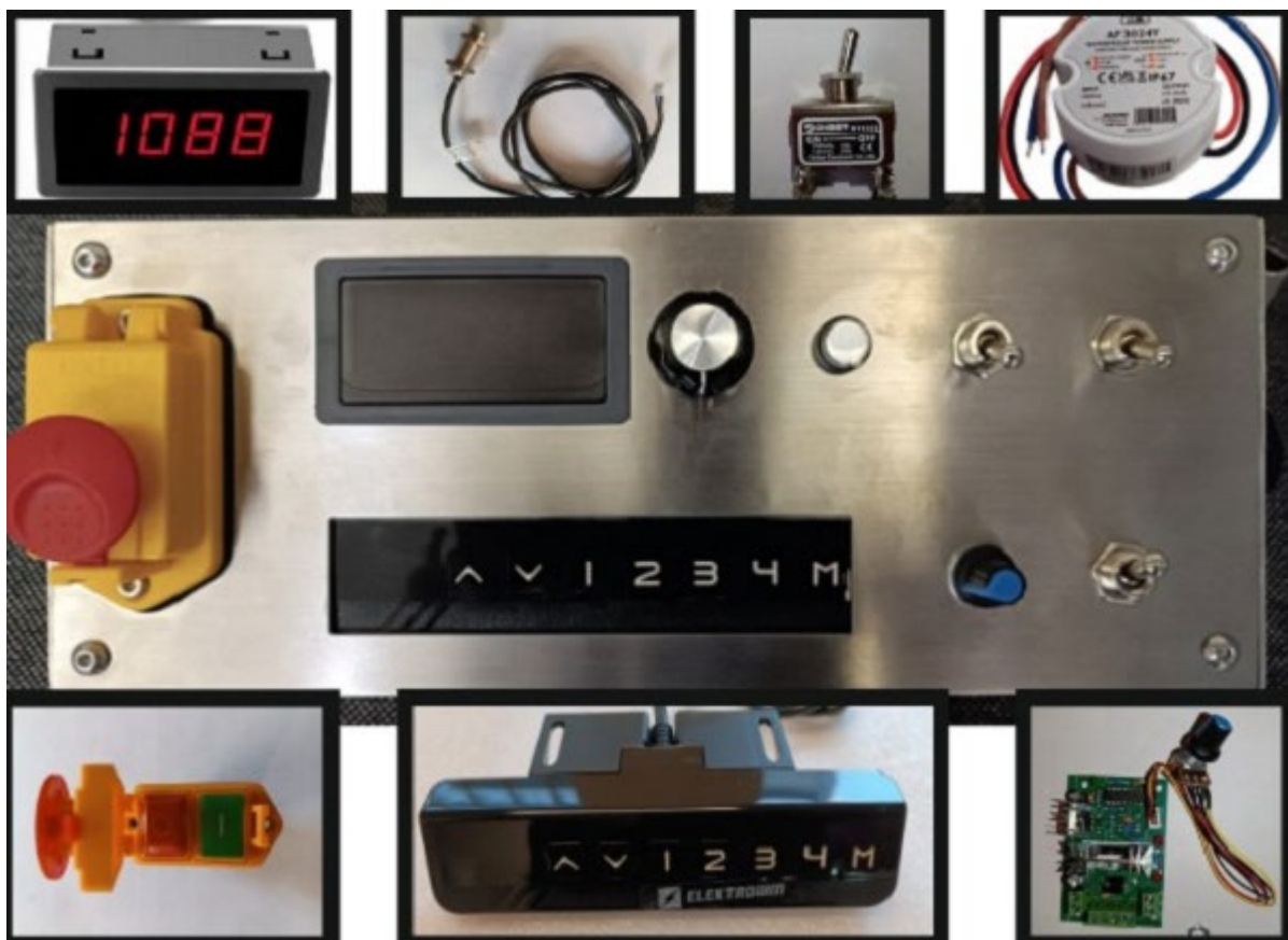
Fig. 52. Assembly of components of the welding table control panel
