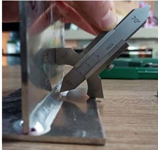
Fig. 6. Method of measuring the weld thickness [239, 240, 241]
