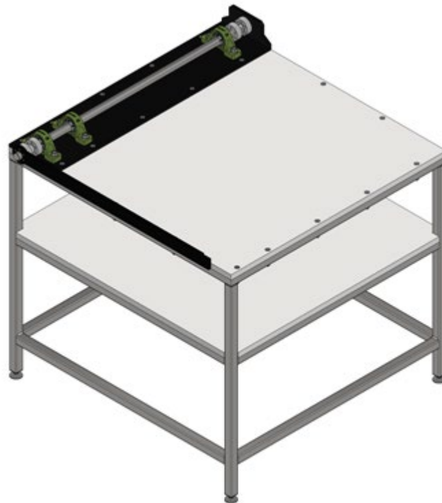
Fig. 25. Model of the test rig for measuring the shaft torsional angle
