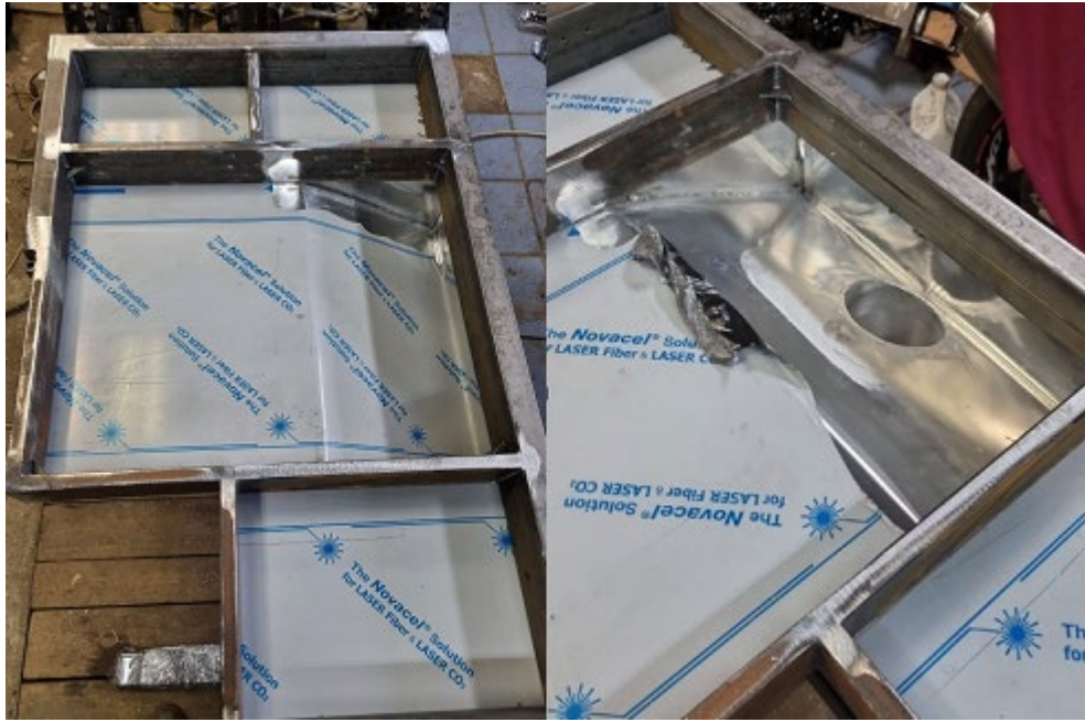
Fig. 37. Table covers made of 1.5 mm thick aluminum sheets
