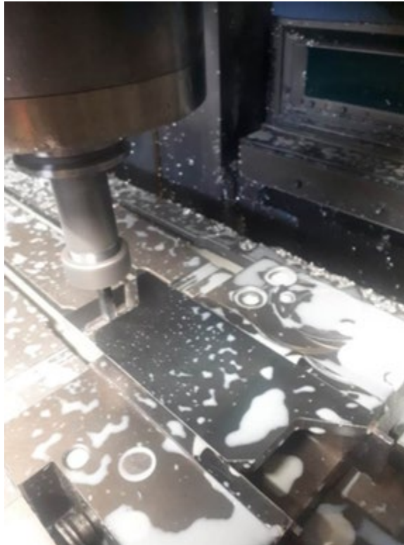
Fig. 32. Finish milling of the shape of the shaft mounting plate
