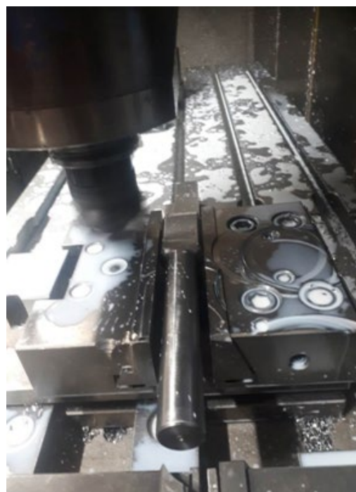
Fig. 36. Milling the sides of the weight mounting pin
