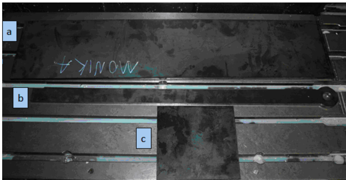
Fig. 26. Laser-cut elements of the test rig for measuring the shaft torsional angle
