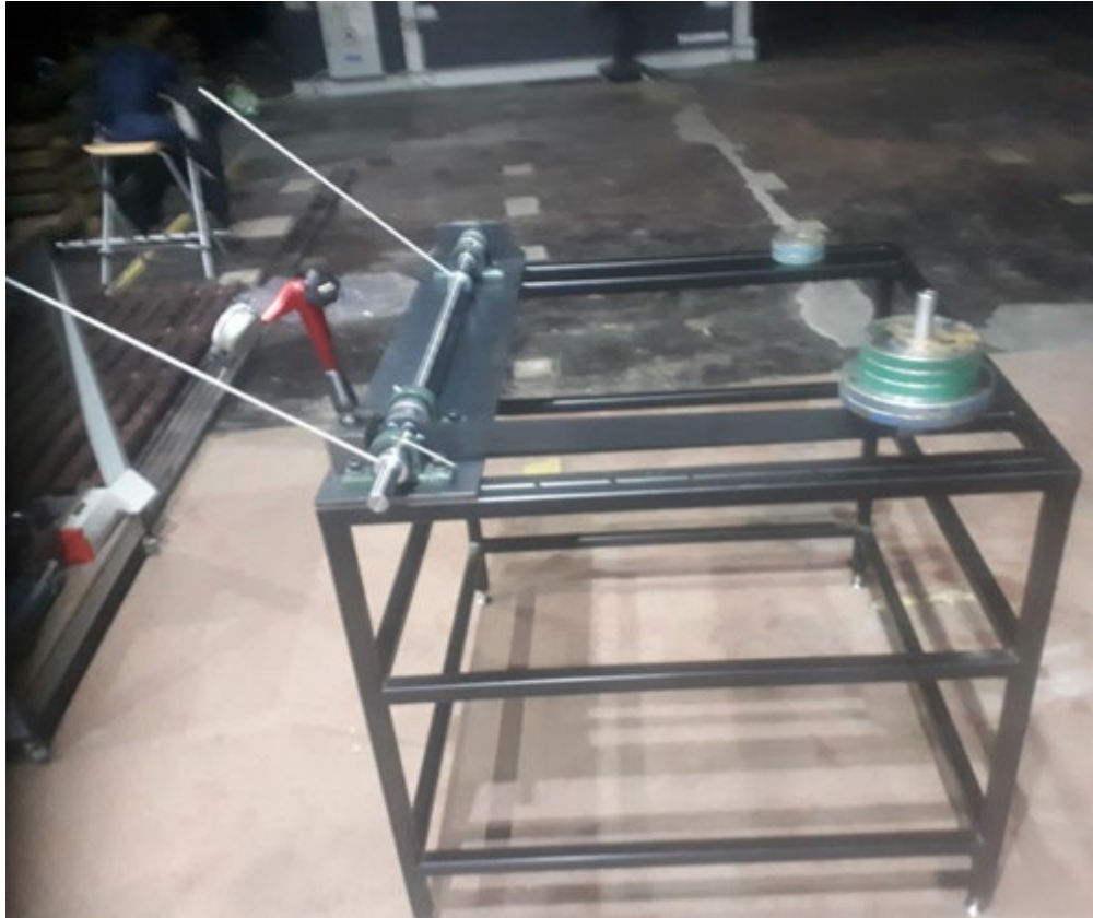
Fig. 43. Test rig for measuring the torsional angle of a uniform shaft with a circular section
