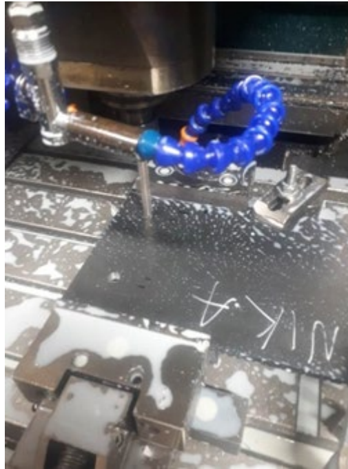
Fig. 28. Drilling \text{\O}12.2\text{mm} holes in the rig plate
