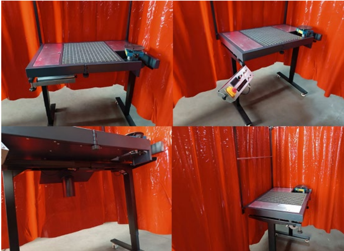
Fig. 53. View of the finished welding table after powder coating (table frame color: graphite RAL 7016, frame color: black RAL 9005)
