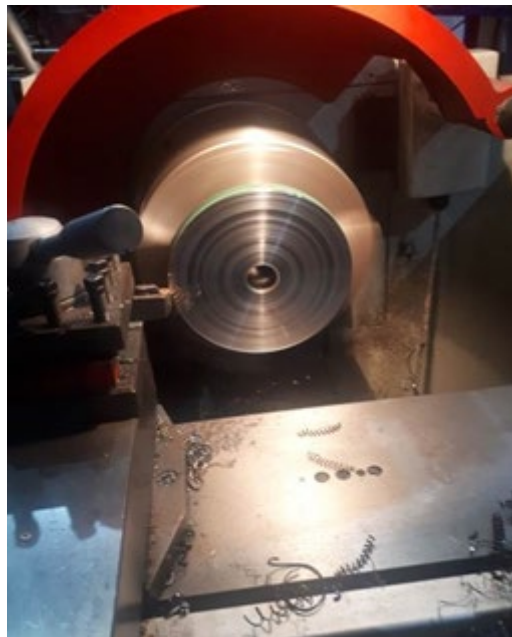
Fig. 38. Turning steel weights on an engine lathe
