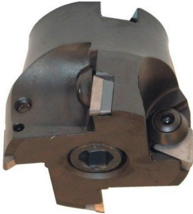
Fig. 20. View of the 80mm TRI-SQ Indexa IND1393420 milling head with SM25T multi-edge inserts
