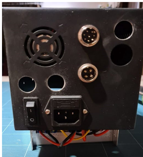
Fig. 9. Hole layout for additional GX16 quick connectors
