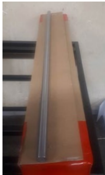
Fig. 40. Linear shaft \text{Ø}25\text{h}6 made of C55 steel
