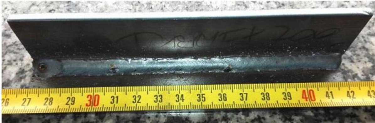
Fig. 2. Example of a sample subjected to visual inspection
