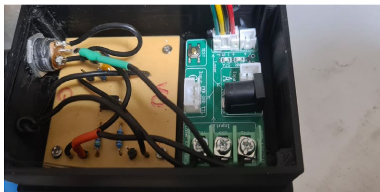
Fig. 19. PWM signal voltage reduction system with laser driver
