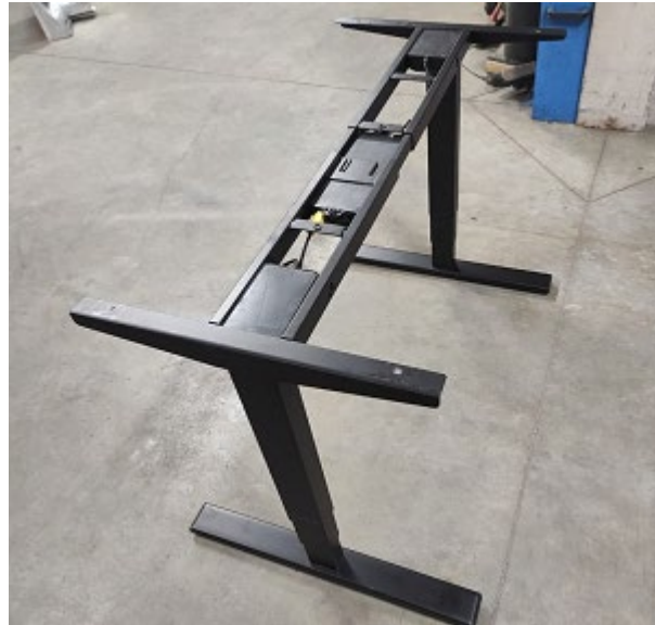
Fig. 38. Commercial ERB-1 frame as a supporting structure for the welding table top
