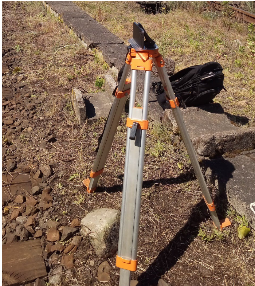
Fig. 9. Aluminum tripod with a mounted phone
