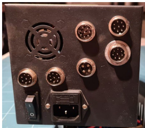
Fig. 13. Location of additional GX16 quick-connect sockets
