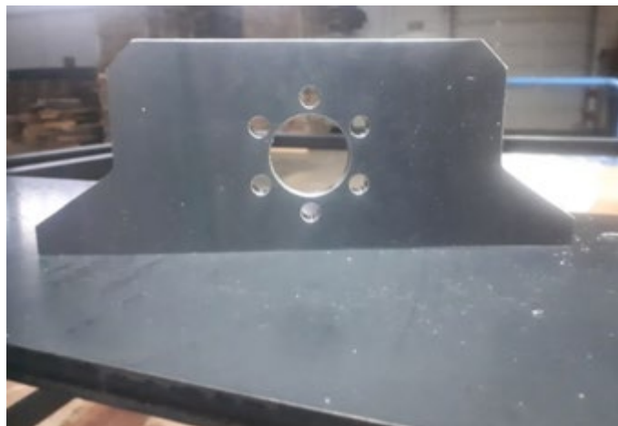
Fig. 33. Back plate for securing the shaft after all machining operations are completed
