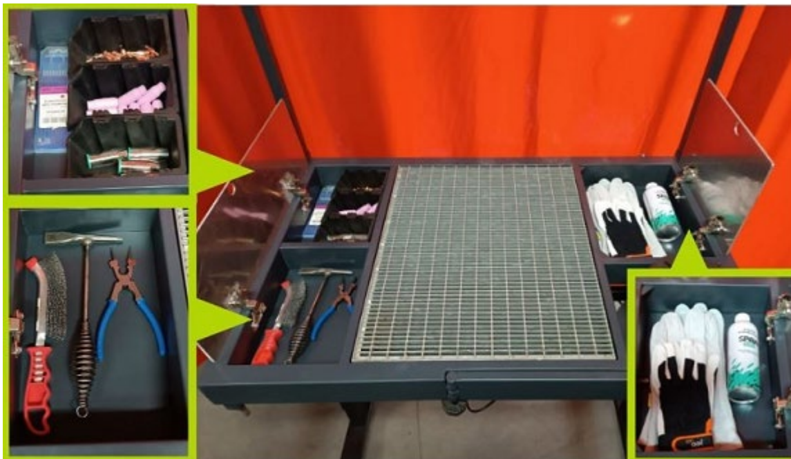
Fig. 56. Example of tool storage arrangement for a designed and constructed welding table
