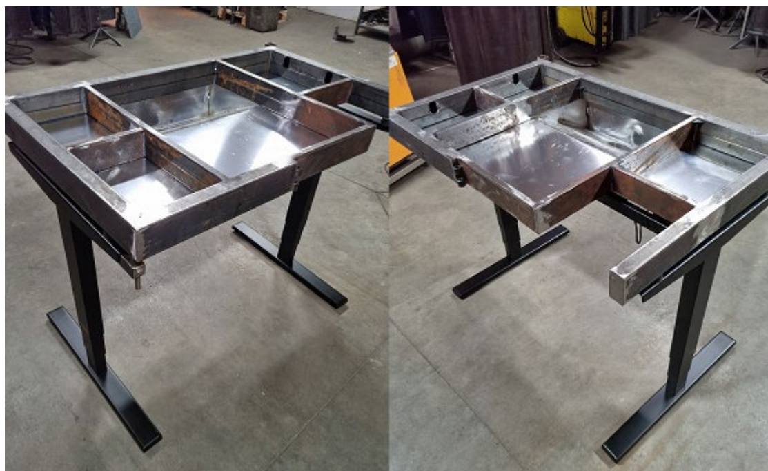
Fig. 40. Mounting the welding table top to the ERB-1 frame
