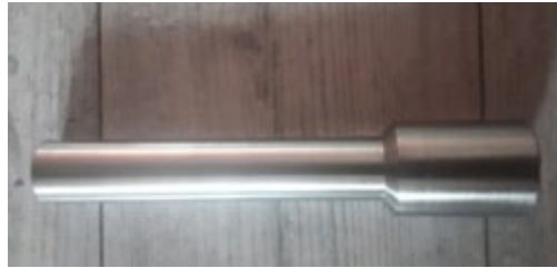
Fig. 34. A weight mounting pin turned on an engine lathe
