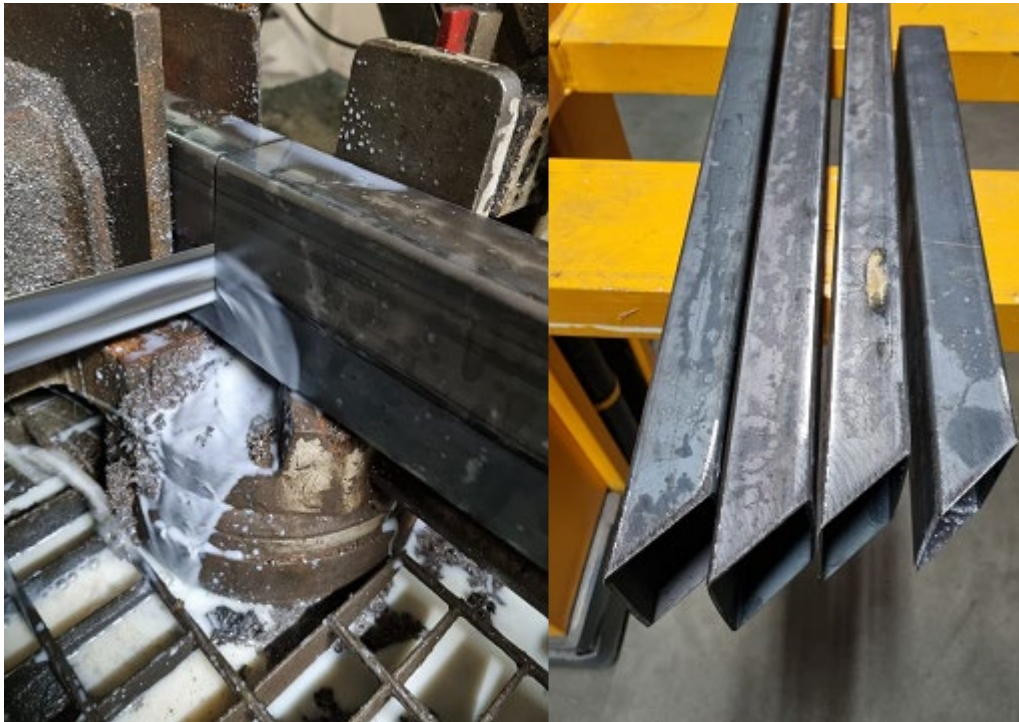
Fig. 29. The process of cutting profiles of the supporting frame of the welding table
