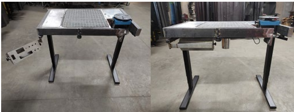
Fig. 47. Mounting the control panel to the welding table structure
