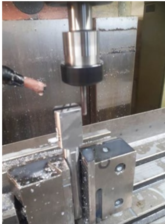
Fig. 35. Milling a groove on the pin, 8.2 mm wide and 42 mm deep
