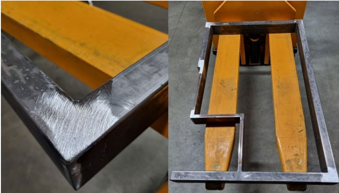
Fig. 32. Welded profiles of the welding table support frame after the process of grinding
