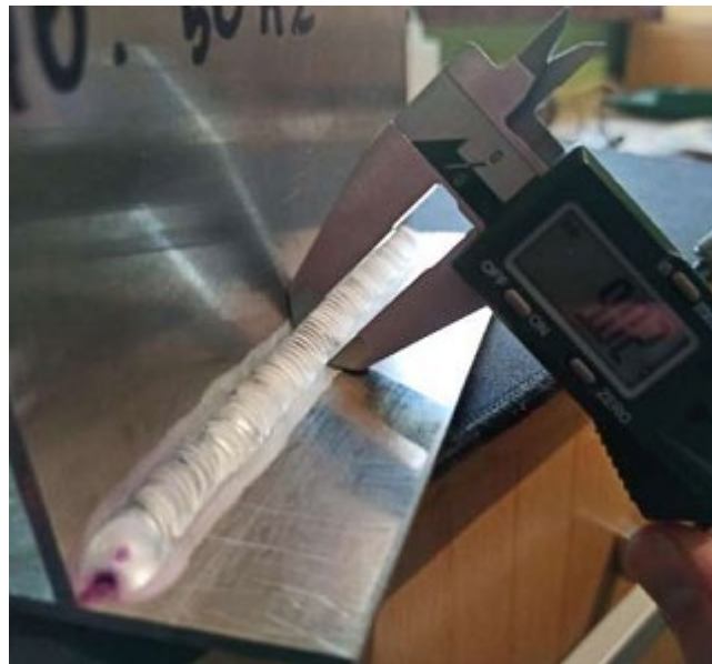
Fig. 5. Method of measuring the weld width [239, 240, 241]
