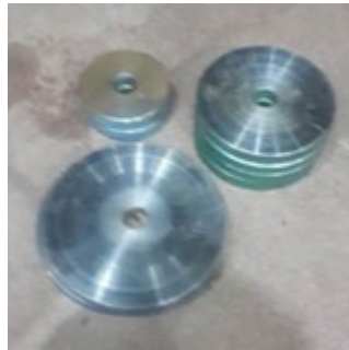
Fig. 39. A set of weights used on the test rig to measure the torsional angle of the shaft
