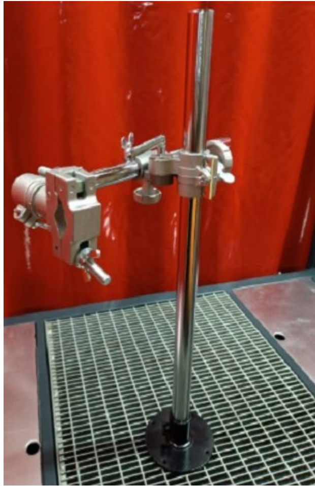
Fig. 26. Welding holder designed for welding in forced positions
