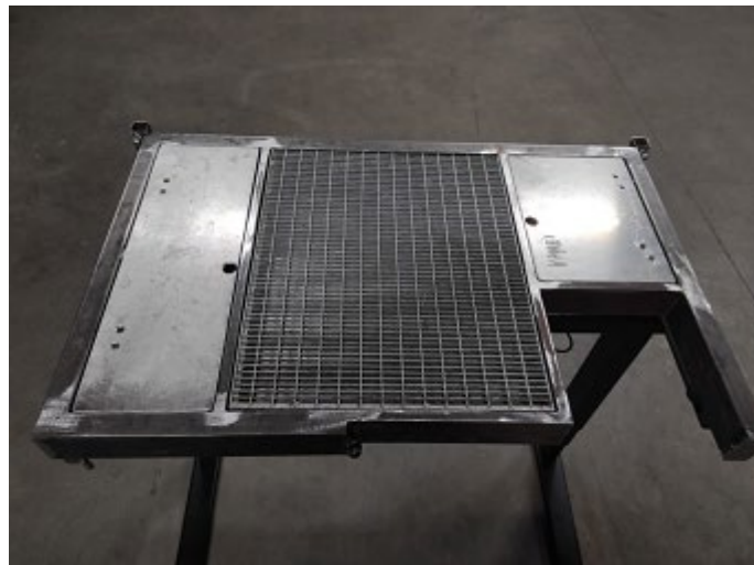
Fig. 43. Assembly of the welding table top truss
