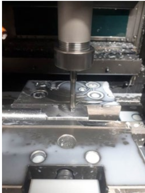
Fig. 37. Making an M8 thread in the side part of the weight mounting pin
