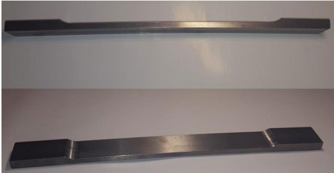
Fig. 16. View of the deformed element after milling
