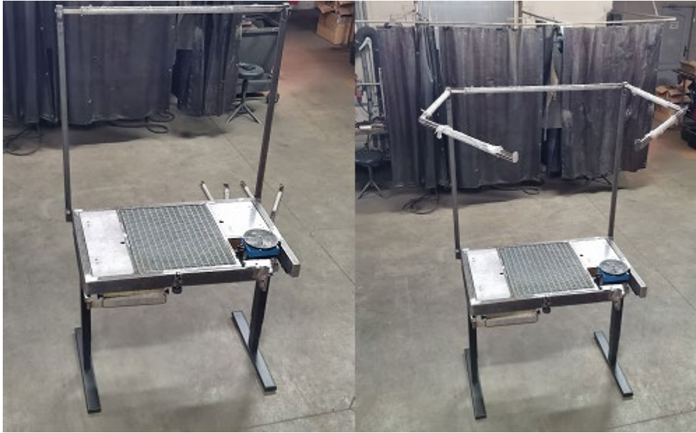
Fig. 49. Installing the protective screen frame for the welding table
