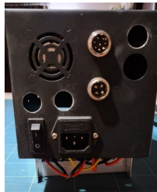
Fig. 12. Additional holes made for mounting GX16 sockets
