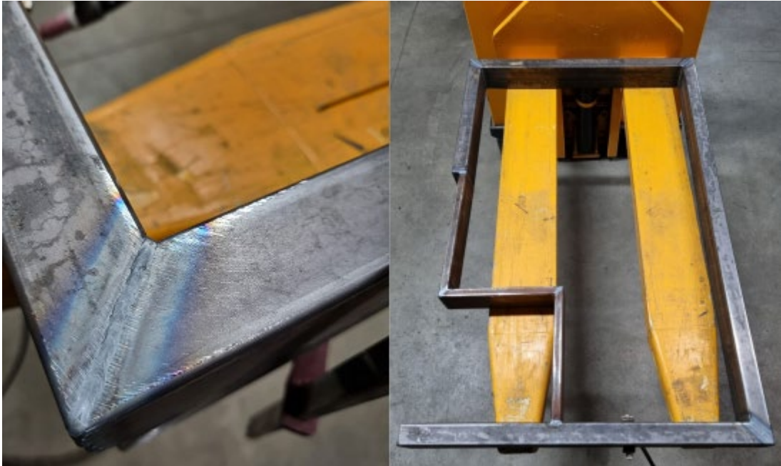
Fig. 31. The process of welding the cut profiles of the supporting frame of the welding table
